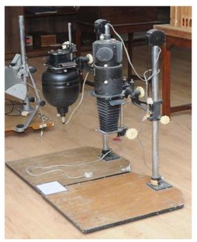
The vertically mounted photo enlarger works by shedding a stream of light down through the negative film to make a photographic print of the image projected onto the enlarger was used extensively by the postgraduate students of the Department of Fine Arts 80's for their course on Photography.
