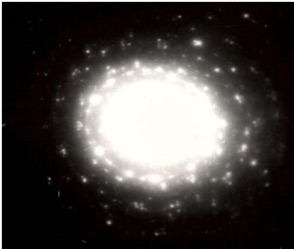
Figure 3: Selected area ED pattern taken from the batch of F4 film on crystallite of size \sim 0.2\mu\text{m} . The pattern clearly indicates the coexistence of several hexagonal crystalline phases having slightly different lattice parameters. Multiple twinning of the crystallites is also evident [17, 21].
