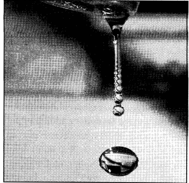
Plateau-Rayleigh instabilities can be observed as a water droplet is formed from a dripping tap
