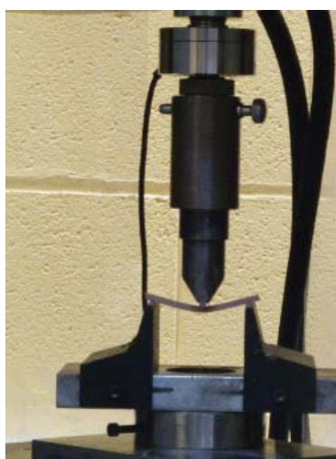
Figure 6.14 A specimen tested in 3-point bending
