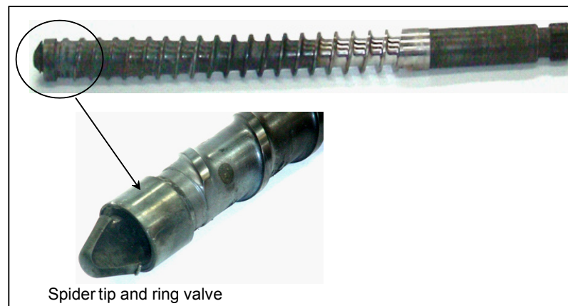
Figure 3.6 Photograph of a typical injection moulding screw and its spider tip and ring valve
