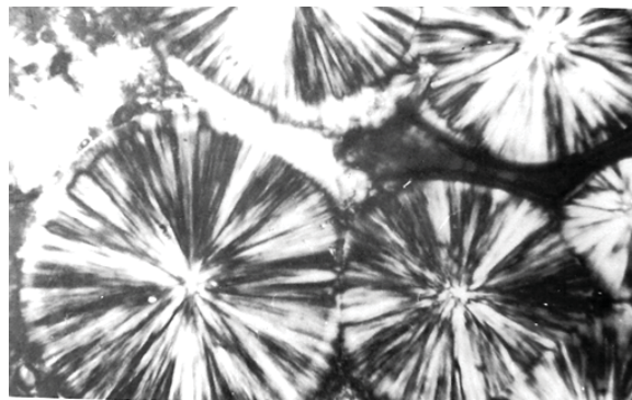
Figure 4.5 An optical micrograph of PP Spherulites
