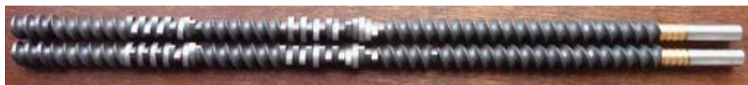
Figure 3.24 Conveyor elements and kneading disks are assembled on the shafts of twin screws
