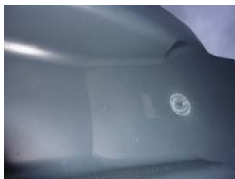
Figure 3.8 The mark left on a large moulding after trimming off the sprue runner
