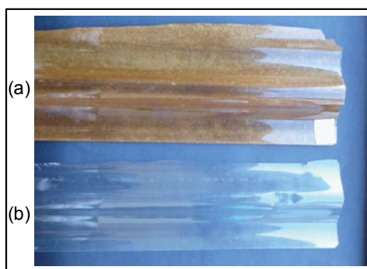
Figure 5.1 Specimens taken from a PVC clear corrugated roof: (a) represents the section of the roof exposed to sunshine, (b) represents the section of the roof shaded from the sun
