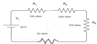
22) Find the Thevenin's equivalent circuit at the terminals x-y of the following circuit.
